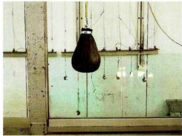
Sample photograph after impact at the midpoint of the upper edge of the glass
